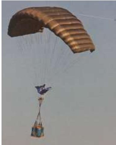
A new innovation in the Aerial Delivery box of tricks is the One-Time Use Guided Precision Aerial Delivery System being tested in the US. This System can be dropped from an altitude of 17,500 feet Above Mean Sea Level (AMSL) and capable of carrying a payload of up to 2,200lbs (a fully loaded A22). The system can glide for up to 25 kilometres and will land within 150 metres of the target.
